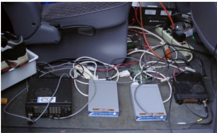
The NG2P packet node demo setup: 2 TNCs, 2 radios, 2 antennas, 2 terminals, miles of wire. And they call this "wireless?"
