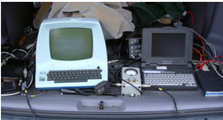
The NG2P packet node demo setup: 2 TNCs, 2 radios, 2 antennas, 2 terminals, miles of wire. And they call this "wireless?"
