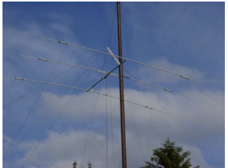
The fruits of the labors. The TA-33 and 80m dipole in place on the flagpole, supported by the famous, patented K1PY GIZMO. Look at all those lines! Wonder where they all go?
