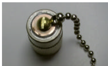
Completed cap with beaded chain attached. This view shows the pipe cap, soldered to the inside of the PL-259 sleeve, and the 6-32 screw holding the beaded chain.
