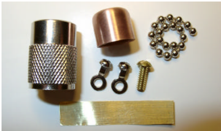
Parts needed to construct a screw-on cap for N and UHF connectors: PL-259 sleeve, 3/8 inch copper sweat pipe cap, 6-32 x 3/8 in. brass machine screw, short length beaded chain and end connectors, brass shim stock.
