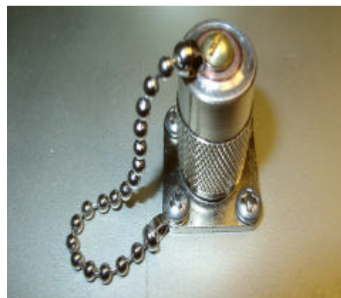
Homebrew connector cap installed on chassis mount SO-239. In this installation, cap has been secured to one of the SO-239 mounting screws to prevent loss when not in use.
