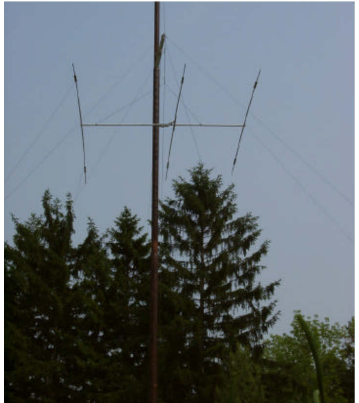
The RDXA yagi; our trusty TA-33 again hangs on the 1939 Boy Scout flagpole, suspended from the K1PY patented GIZMO-1. This gets easier every year!
