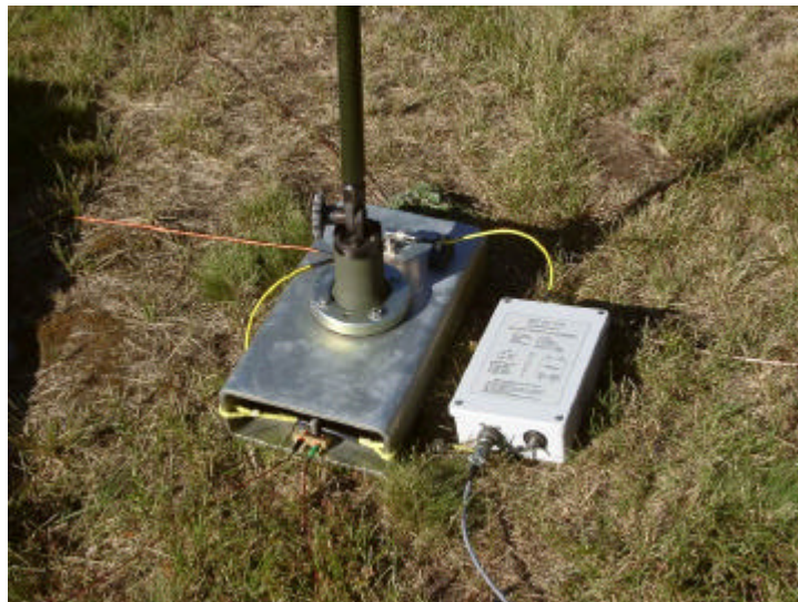
The base of the whip is mounted on a short piece of 10-inch steel channel stock. This 60 pound "counterweight" makes the antenna freestanding. Antenna feed was via an SGC 237 autotuner in a homebrew weathertight case. Five, 32 foot radials were deployed as a ground system.
