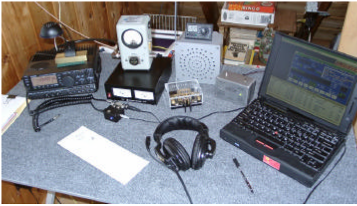
The shack on the new table: FT900, Astron switching power supply, Bird 43 and logging computer. This operation was the first with the SGC 237 autotuner and the Bird provided a means to closely observe the matching.
