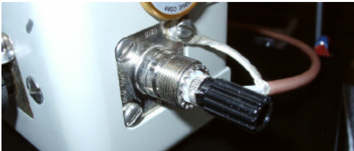
Temporary coax hookup via a standard binding post to the output connector on the Bird 43. A chassis mount binding post with 8-32 threads fit perfectly into the center contact of the SO-239. The coax braid was tinned and attached to one of the mounting screws of the UHF connector on the Bird.
