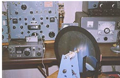
The receiving end at the AWA Museum showing the modified Kenwood R-1000 receiver and the “televisor” – a mechanical disk scanner and magnifying apparatus. [AWA Photo]
