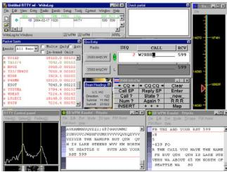
A very useful utility, F-Keys, in the center of my screen allows user programmable Function Keys to automate common messages such as sending CQ and asking for repeats with just a click. It is also used for CW and Phone contesting.
