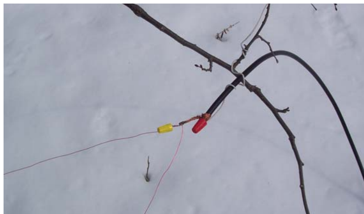
Picture 2: Inverted L feedpoint with unique wire nut attachments.
