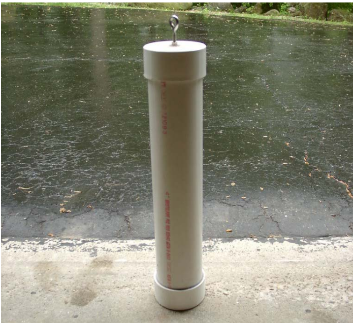
A PVC counterweight, filled with sand and nails. Height is about 3 ft. Works great but it's ugly; stands out like a sore thumb hanging in the yard.
