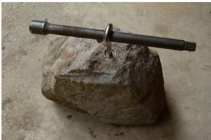
Installing the screw eye in the lag shield A cheater bar is essential.
