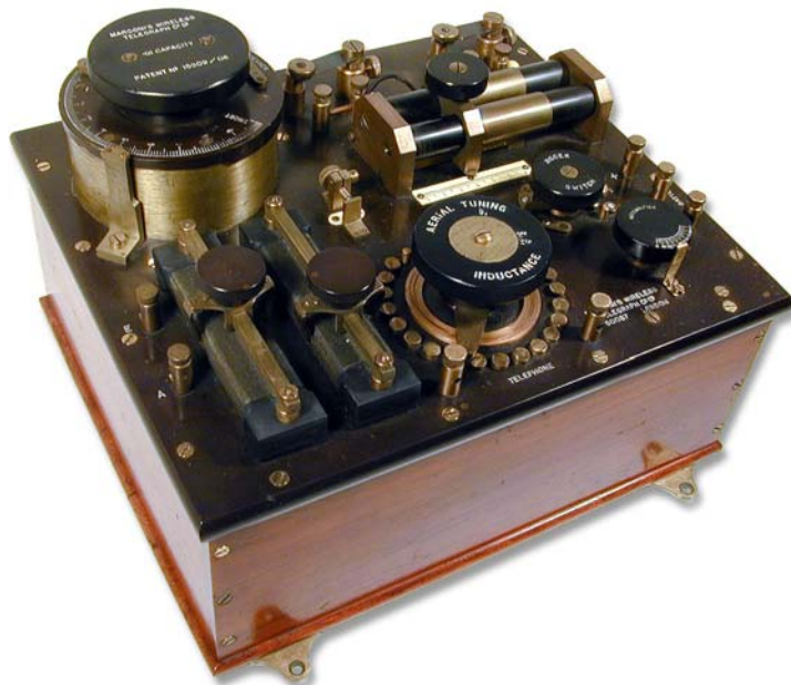
Marconi Model 16 Balanced Crystal Receiver, ca. 1916.
