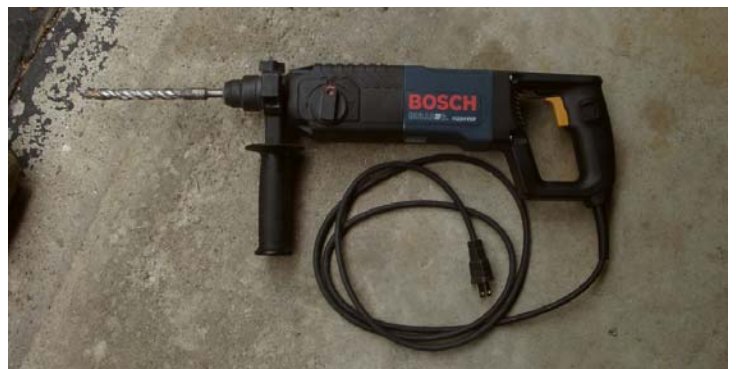
The Bosch Bulldog hammer drill. Bores through granite, concrete, brick, concrete block, slate, asphalt—you name it—like a hot knife through butter.
