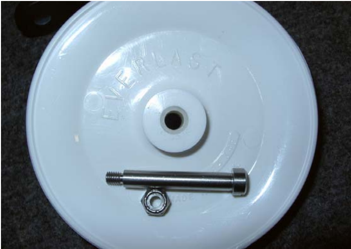
A stainless steel shoulder bolt and nylon insert locknut, for making a pulley with removable sheave from Everlast #50 components.
