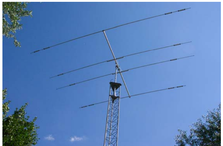
A thing of beauty. The Mosley TA-53 installed, tuned and ready for rare DX.
