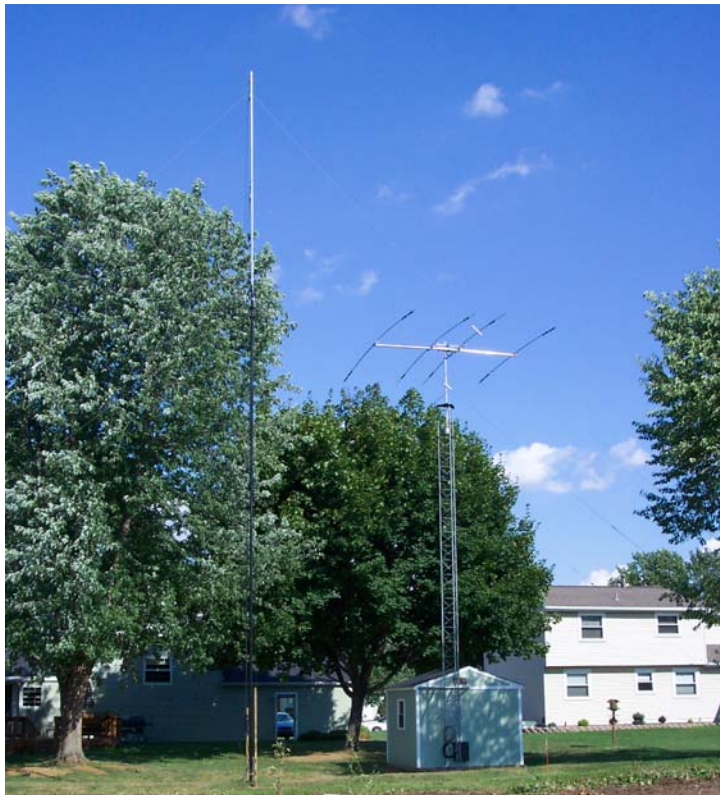
The complete installation at WB2HJV; a new yagi and effective low band inverted VEEs. Watch out for this guy in the pileups this winter!
