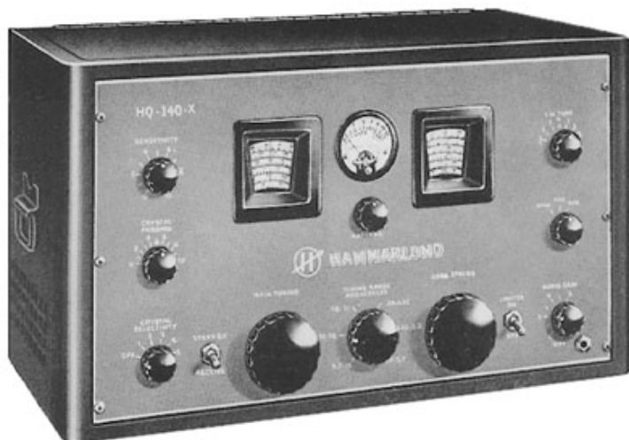
The Hammarlund HQ-140-X general coverage receiver, with bandspread for 80-10m ham bands. Single conversion superheterodyne, 11 tubes, AM/CW.
