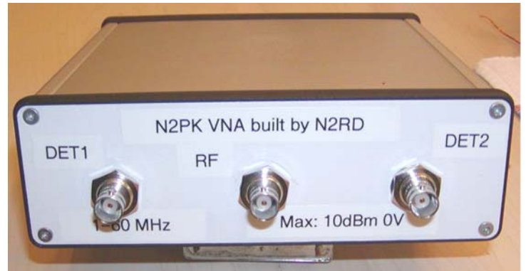
N2PK Vector Network Analyzer built by N2RD.
