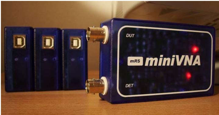
Mini-VNA from mini Radio Solutions. Adequate for antenna measurements.
