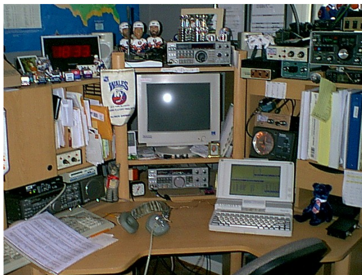
Chris, K2CS: The K2CS station is comprised of a TS440SAT, MFJ keyer, a spare TS440 to the left, an FT620B for 6m, top right, and in the center a TS711 for 2m weak signal. The 2m and 6m bricks are on the right top. The antennas are a C3 with the infamous G5RV. DOS-based laptop for logging.
