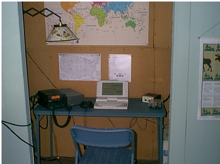
Coldbrook Contest Club, W2CCC: K2CS trustee. TS50, matching autotuner, power supply and MFJ keyer (with the W2OMV benchner), that's it! Outside is the W2OMV Butternut vertical and a 160m dipole. Another DOS-based laptop is used for logging at W2CCC.
