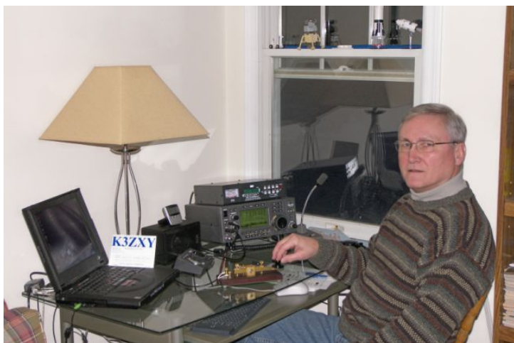
Wayne, K3ZXY: Wayne's compact setup includes a TenTec Pegasus rig, with an LDG autotuner and a classic, long-arm straight key.
