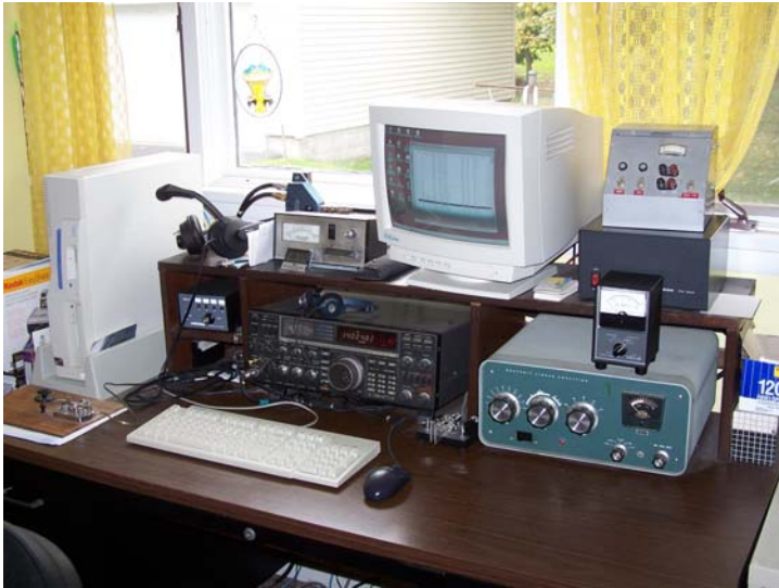
The neat operating position in Dave's shack sports an IC-765 with 250Hz filters and the venerable Heathkit SB200 linear amplifier.
