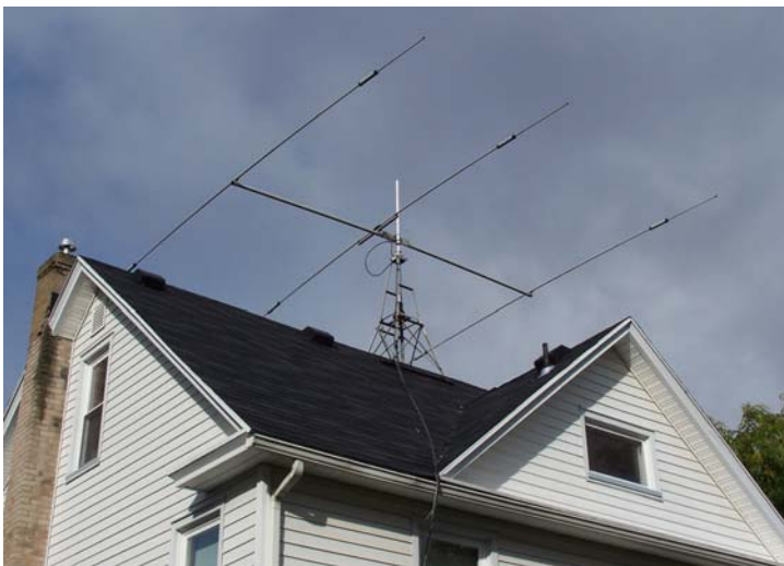
At the other end of the coax: a Mosley Classic TA-33 tribander, with plenty of room on the mast for another antenna, yet to be determined.
