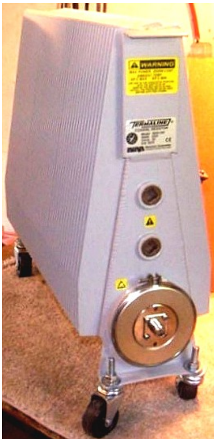
The Radiator...er, dummy load used for amplifier testing and tuning.
