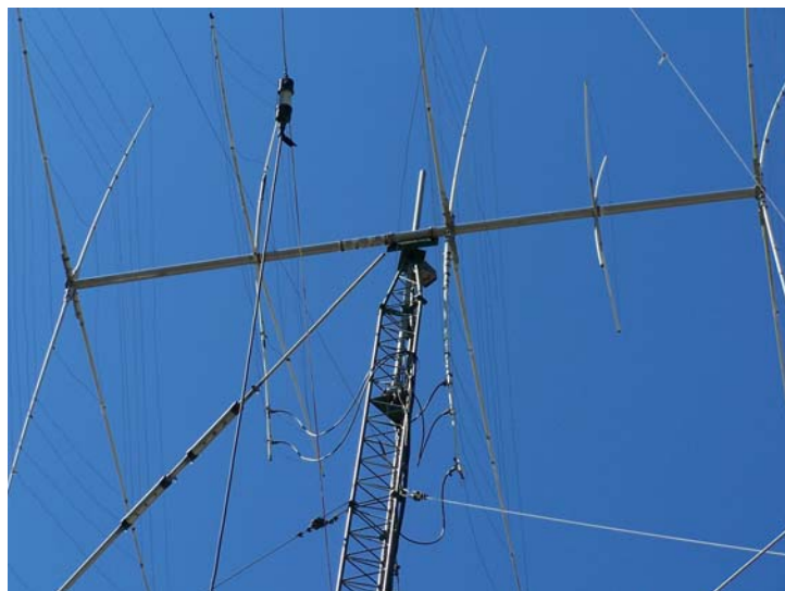
Closeup of the quad antenna at TI5N. Note the multiple feedlines and multiple loops on each element. This really is a custom antenna.
