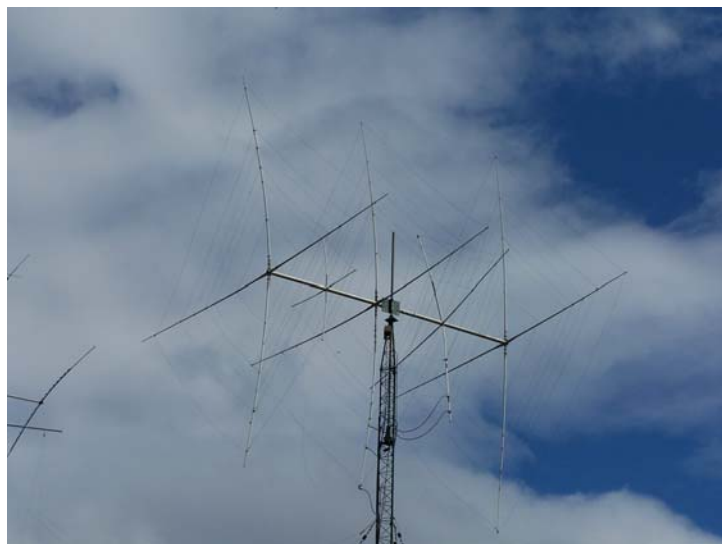
The star antenna at TI5N: a homebrew 4-band, 4 element quad.
