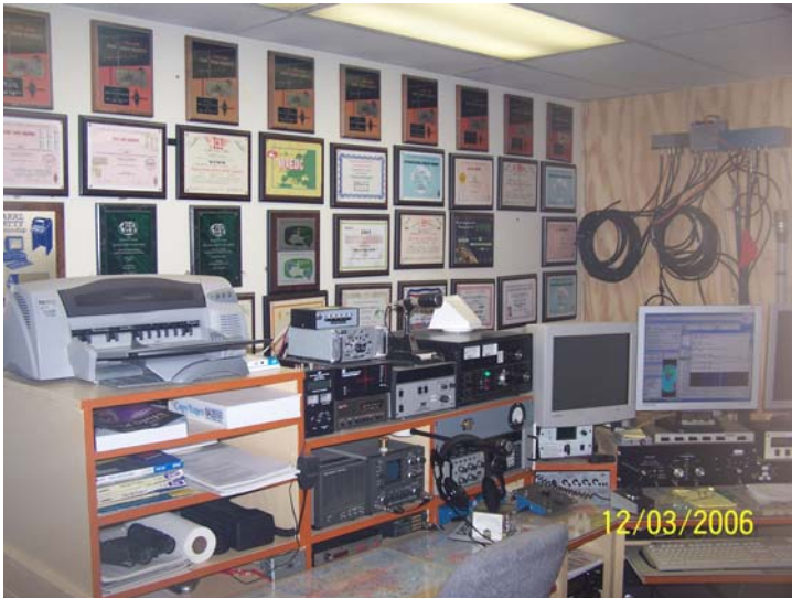
Operating position 1 at N2WK features a Ten Tec Omni VI and a modified Dentron amp.
