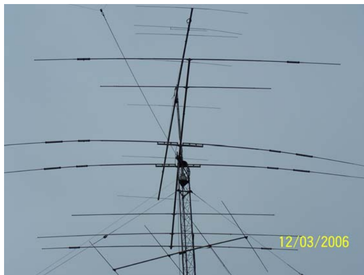
Tower #3 Rohn 25G , 70 feet. 7el 6m Cushcraft @ 80 ft.; Mosley Pro 67A @ 70 ft. 10/12/15/17/20/40m, 4el on 10m, 3 on other bands and 2 el on 40m; the tower also supports an 80m sloper.
