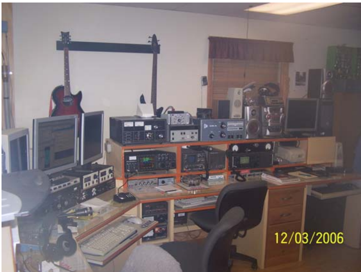
Operating position 2 (center) at N2WK includes the Ten Tec Orion II and another modified Dentron amp. Operating position 3 (right) features an Icom 746 Pro and an Alpha 86 amp for 6m only.
