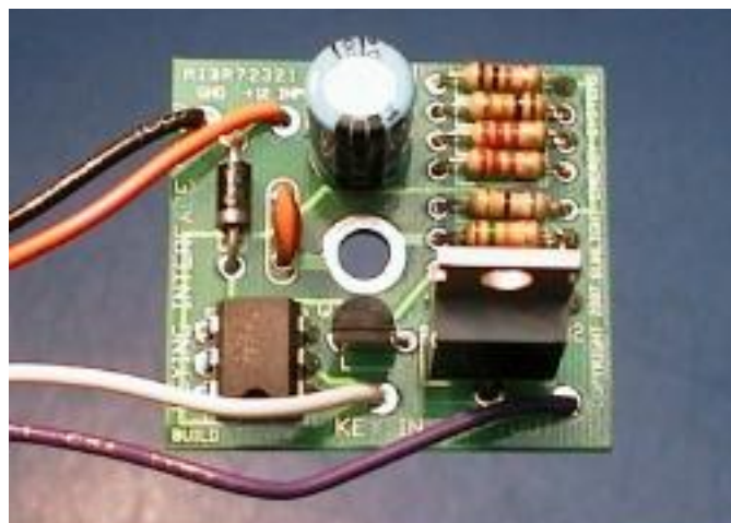
WB8VGE Universal Keying Interface. The LED indicator is not visible. It's behind the electrolytic cap. http://www.theheathkitshop.com/index.html
