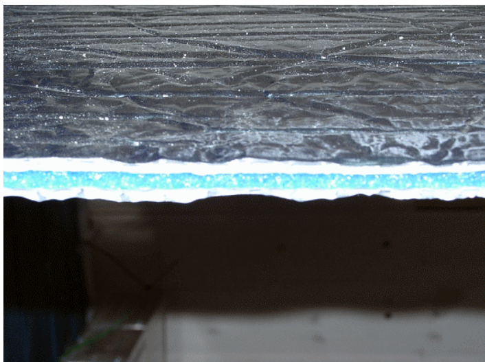
High-efficiency insulation used in the new OZ5E shack is a sandwich of closed cell foam and bubble-wrap like material made with aluminized plastic. Thickness is only 15-20 mm.
