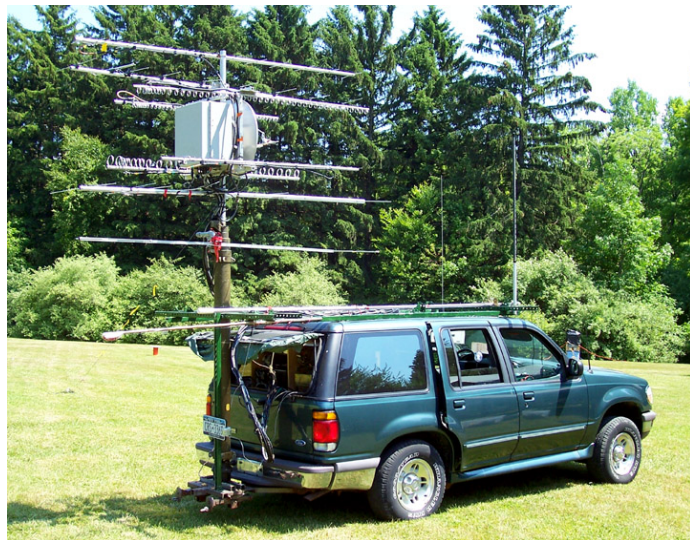
Rover vehicle of Bill Rogers, K3TER/R ; beams used for VHF/UHF station in FD.
