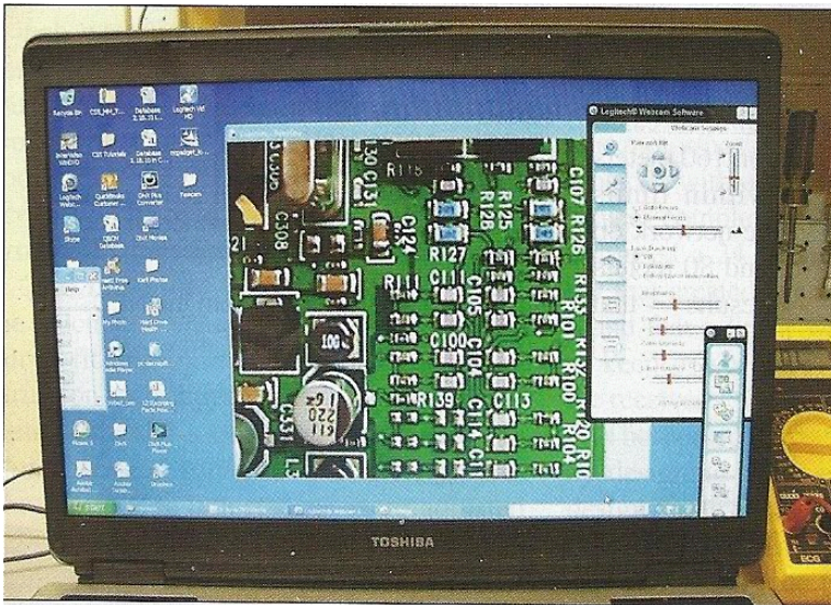
Figure 2 — The laptop screen showing a portion of the PCB with the tiny surface mounted components.
