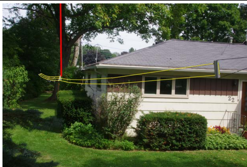
FIGURE 3 OVERVIEW OF THE 160M FCP. ENHANCED TO SHOW THE FCP WIRES IN YELLOW AND THE BASE OF THE INVERTED V IN RED.
