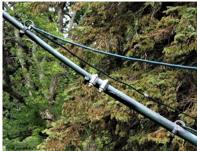
Split hexbeam arm repaired with hose clamps two years ago is still holding well
