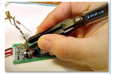
tinuous use. It goes to sleep to preserve power after 60 seconds of no motion and wakes up in a couple of seconds when you pick it up.
