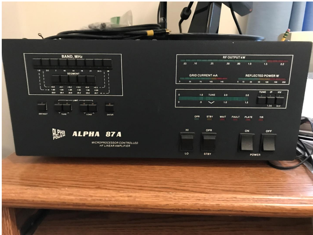
Fig. 2: The Alpha 87A on a desk at WA2CHV. Note the lack of “TUNE” or “LOAD” control knobs on the front panel. The TUNE and LOAD capacitors are adjusted via stepper motors and front-panel switches.
