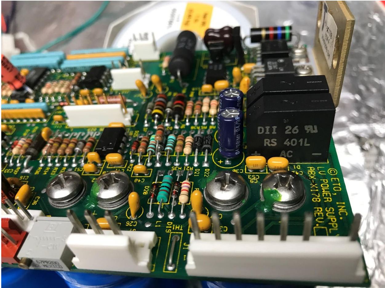
Fig. 8: The failed RS 401 L on the low voltage power supply board.
