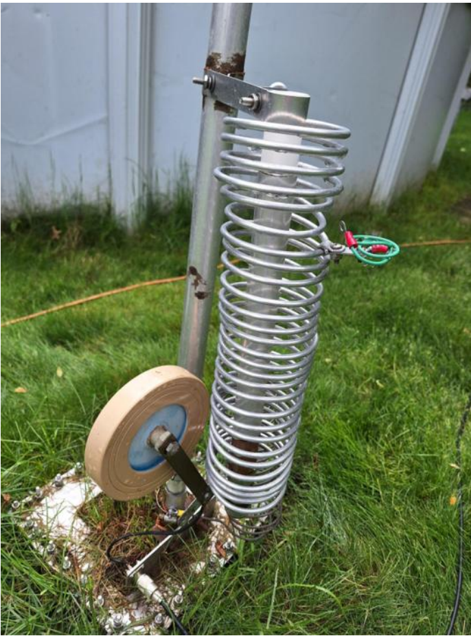
Figure 2- Base of Butternut HF2V with TBR-160 Kit in Place with Replacement 400pf Cap, Coil Tap Disconnected
