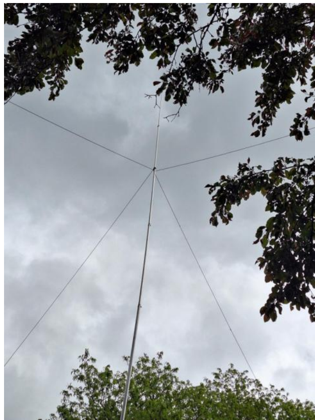
Figure 1- The Butternut TLK Top-Loading Kit
